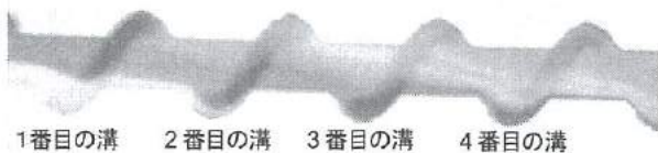
図9 らせん溝部の混合状態( y_d=50\mu\text{m} , s_d=100\mu\text{m} ) Fig.9. Micro Channel Mixing
