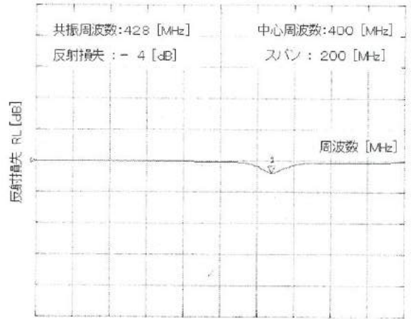
図10 反射損失の測定 (Px=Py=75mm, Fy=15mm) Fig.11. Measuring of the RL characteristic. (Px=Py=75mm, Fy=17.5mm)
